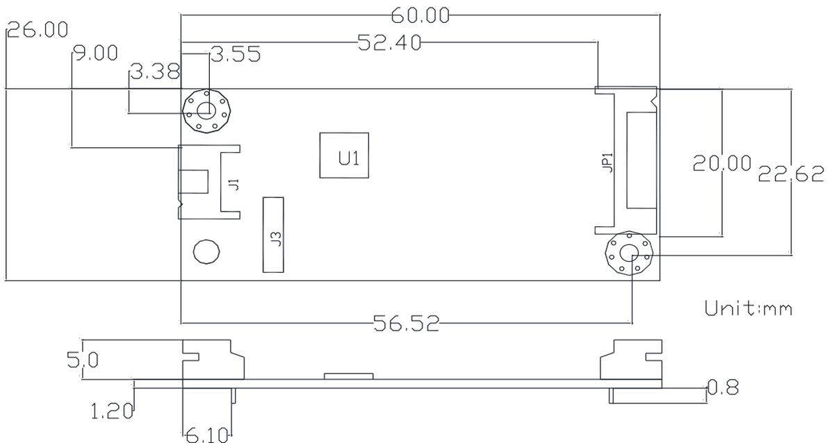
**PM6300A5** supports 5 wires touch panel, R12 is not mounted in the circuit.
