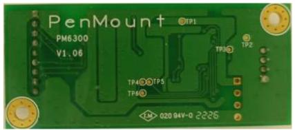
PM6300B8 supports 4/8 wires touch panel, R12 is mounted in the circuit.
