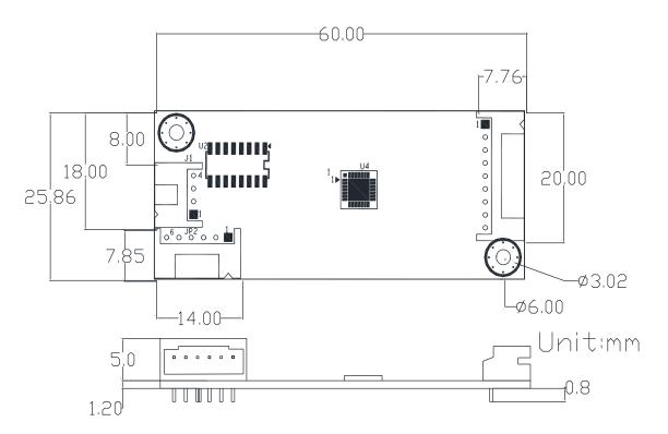
**Mechanical Size** : PM6500A5 and PM6500A8 are the same mechanical size.
