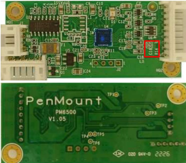
PM6500D8 supports 4/8 wires touch panel, R14 is mounted in the circuit.
