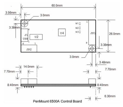
**PM6500A5** supports 5 wires touch panel, there's a 0 ohm resistance of R14 in the circuit- therefore we don't mount the component.
